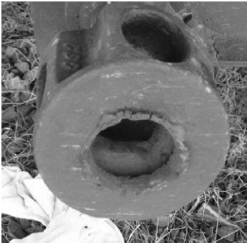
Damaged capstan (rounded square drive socket)
