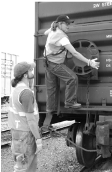
3-point Contact for applying a vertical handbrake
