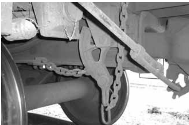
Bell crank in released position
